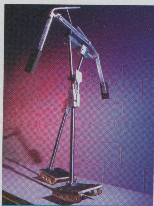
PASSIVE PROMENADE — Swinging its limbs in response to gravity’s pull, this walker built at Cornell University strides down a slope without using a single motor.
